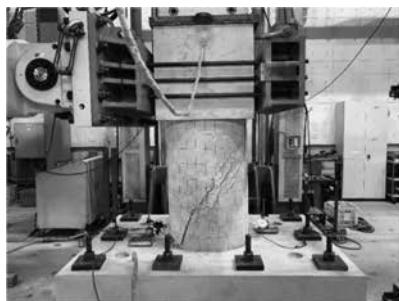
図5 No.3試験体の損傷状況 ( $4 \delta_y$ 、引き側)
