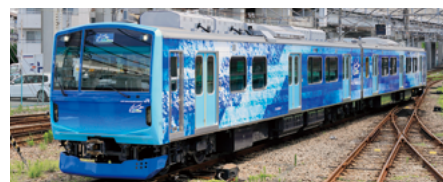
Hydrogen hybrid train, HYBARI (FV-E991 Series)
