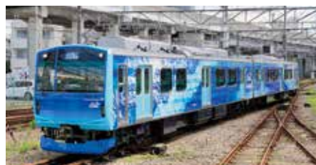
Hydrogen hybrid train, HYBARI (FV-E991 Series)
