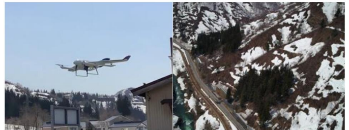
Utilization of VTOL drones for survey operations in the event of a disaster and emergency Scheduled to be used for winter avalanche slope surveys (on a section of the Joetsu Line) starting in the winter of 2026
