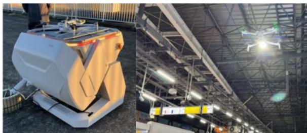
Early detection of defects using drones taking off from drone docks installed along the tracks Scheduled for a trial introduction on the Yamanote Line starting in the fall of 2026
