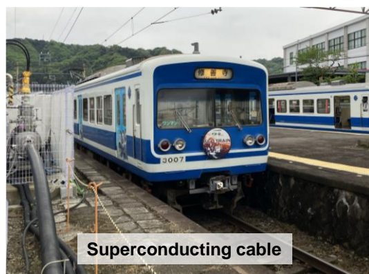
Fig. 1: Train running through power supply section using superconducting feeding system (long-term operation on Sunzu Line)
