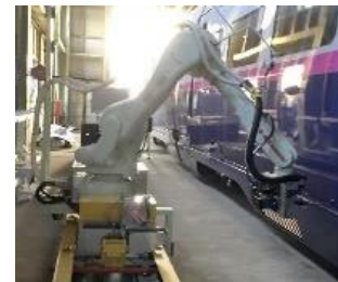
Equipment for automatic dismantling of side cover boards
