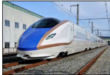
E7 series (2015) VVVF inverter control Regenerative brake
