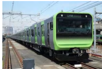
E235 series (2015) VVVF inverter control Regenerative brake
