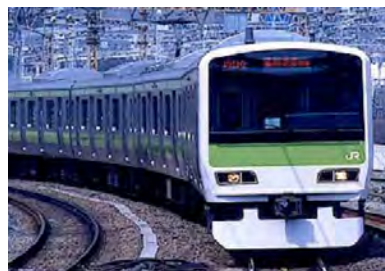
E231 series (2000) VVVF inverter control Regenerative brake
