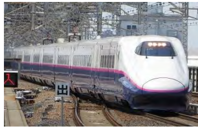
E2 series (1997) VVVF inverter control Regenerative brake
