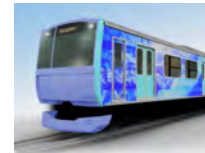
Fuel-cell test railcar that uses hydrogen energy
