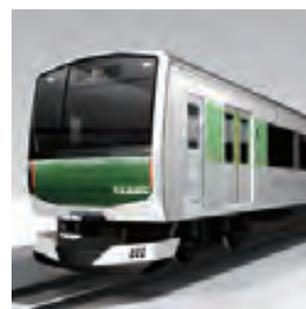
Catenary and battery-powered hybrid railcar train
