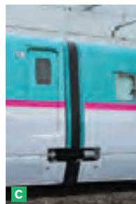
To hold down the noise from operating at high speeds, the pantographs of JR East's latest Shinkansen railcars are fitted with **sound blocking panels A** on both sides. In addition to this, the equipment underneath the railcar floors is covered with sound-absorbing panels, and the gaps between railcars have **canopies completely sealing them B C**.
