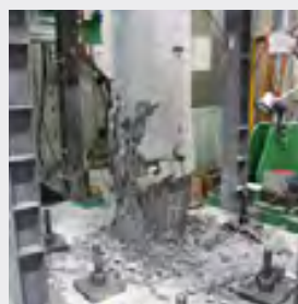
Damage to a pole without reinforcement
