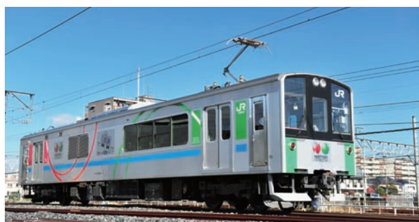
A catenary and battery-powered hybrid railcar
