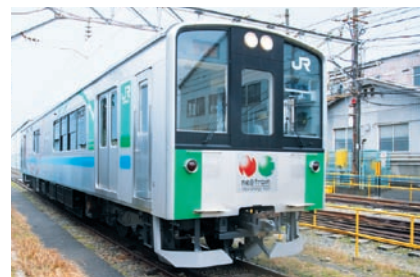
Test runs started with the world's first fuel-cell hybrid railcar
