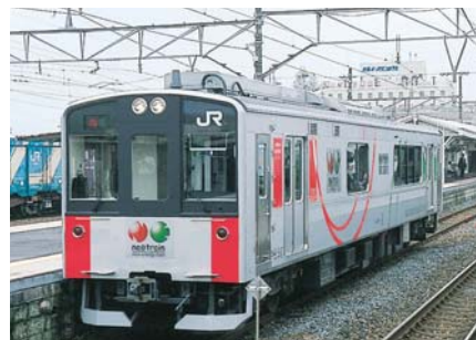
Hybrid railcars that employ fuel cells
