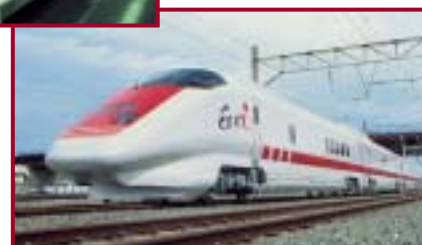
East-1 This next-generation integrated electrical testing vehicle operates on Shinkansen tracks. It handles tasks that previously had to be performed manually, such as track inspections and testing of contact wires.
