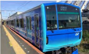
Fuel cell hybrid train, HYBARI
