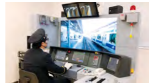
A simulator brings the crew-member training experience to life using actual video footage
