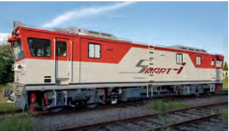
The SMART-i dedicated maintenance railcar with Shinkansen track equipment monitoring systems for Shinkansen Lines has been introduced on a trial basis.
