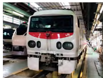
East-i is an electricity and track general inspection railcar equipped with overhead wire equipment monitoring systems.
