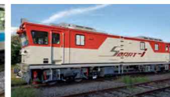
The SMART-i dedicated maintenance railcar features Shinkansen track equipment monitoring systems for Shinkansen Lines.
