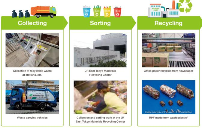
\* RPF (Refuse derived paper and plastics densified fuel): High-grade solid fuel from used paper and waste plastics mainly in industrial waste
