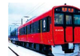
EV-E801 series Accumulator railcar train for use on alternating current (AC) section
