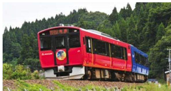
The EV-E801 Series is a new type of battery electric multiple unit train that can run in AC-powered sections and non-powered sections.
