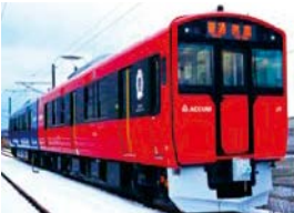
EV-E801 series Accumulator railcar train for use on alternating current (AC) section
