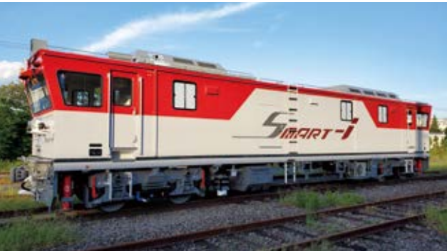
The SMART-i dedicated maintenance railcar features Shinkansen track equipment monitoring systems for Shinkansen Lines.
