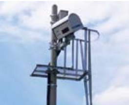
Three-dimensional laser radar obstacle detector
