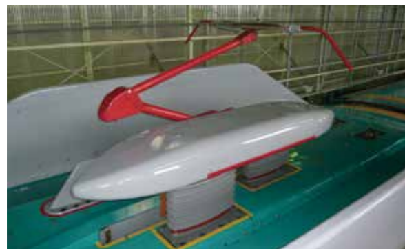
E5 Series trains have low-noise pantographs
