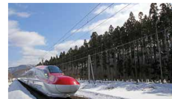
Sashimaki No.1 railway forest on the Tazawako Line (forest to protect against blizzards)
