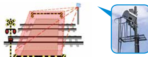
Three-dimensional laser radar obstacle detector
