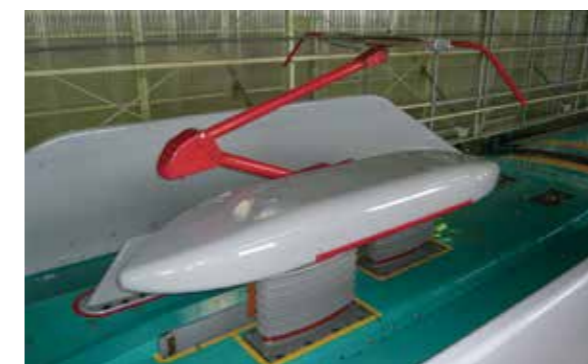
E5 Series trains have low-noise pantographs
