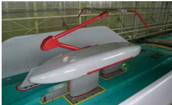
E5 Series trains have low-noise pantographs
