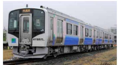
HB-E210 series: Diesel-powered, electric-motor-driven hybrid railcars
