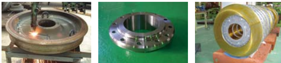
At Nagano General Rolling Stock Center, retired wheels are recycled into brake disk parts
