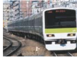
E231 series: VVVF inverter cars for commuter and suburban transportation
