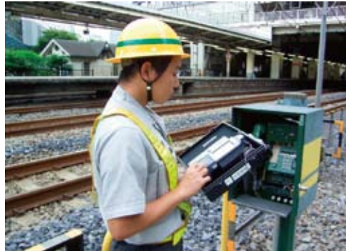
Track closure procedure by a handheld device for maintenance work
