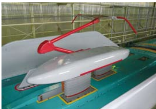
The E5 Series employs low-noise pantographs.
