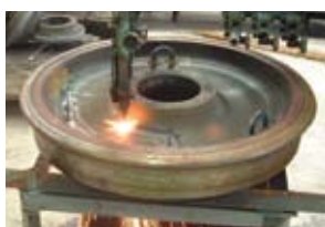
At Nagano General Rolling Stock Center, retired wheels are recycled into brake disk parts.
