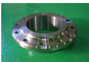
At Nagano General Rolling Stock Center, retired wheels are recycled into brake disk parts.
