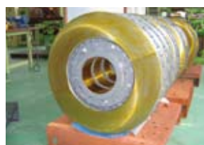
At Nagano General Rolling Stock Center, retired wheels are recycled into brake disk parts.
