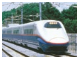
E2 series VVVF inverter railcars used for Shinkansen "Asama" and "Hayate" trains.
