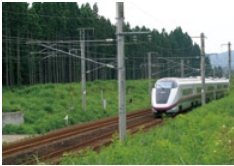
Jinguji No. 2 railway forest on the Ou Main Line (forest to protect against blizzards)
