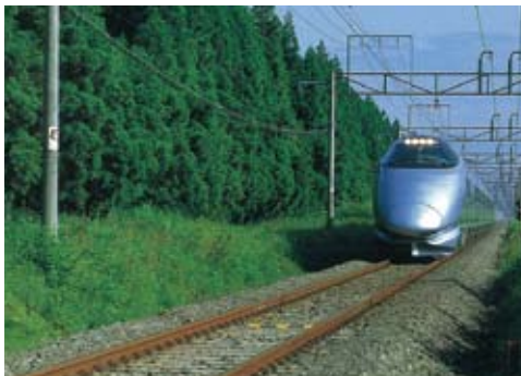
Sekine No.1 railway forest on the Ou Line (forest to protect against blizzards)
