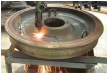
At Nagano General Rolling Stock Center, retired wheels are recycled into brake disk parts.
