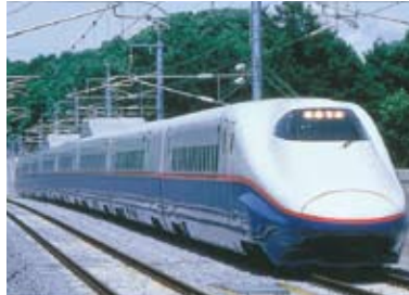
E2 series: VVVF inverter railcars used for Shinkansen "Asama" and "Hayate" trains.
