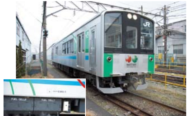
Test runs started with the world's first fuel-cell hybrid railcar.
