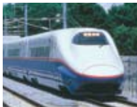
E2 series: VVVF inverter railcars used for Shinkansen "Asama" and "Hayate" trains.
