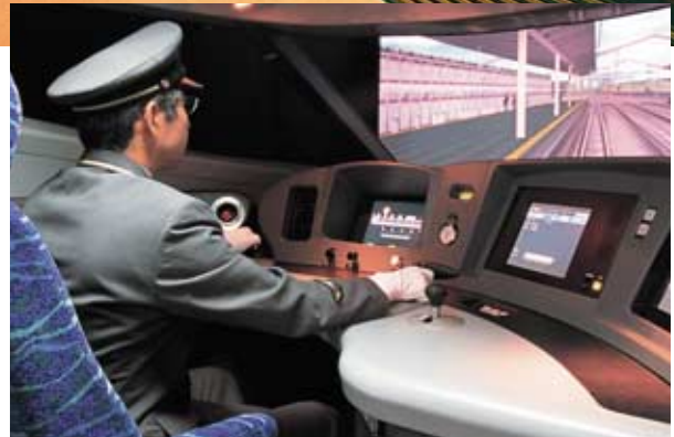
Shinkansen operator training simulator that conducts accident prevention training
