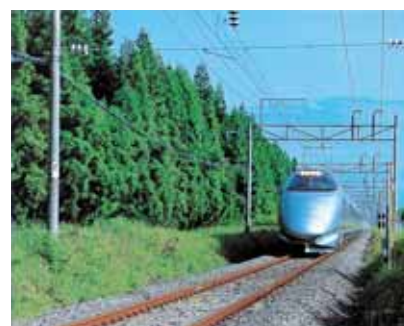
Trees along the JR East Ou Line prevent snowdrift build-up. Shown here is the Yamagata Shinkansen.
