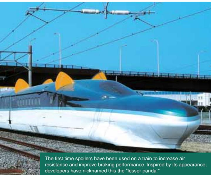
The first time spoilers have been used on a train to increase air resistance and improve braking performance. Inspired by its appearance, developers have nicknamed this the "lesser panda."
