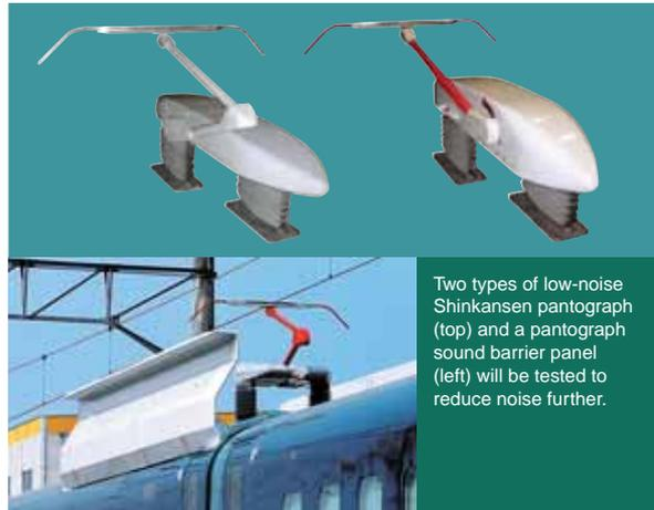
Two types of low-noise Shinkansen pantograph (top) and a pantograph sound barrier panel (left) will be tested to reduce noise further.
