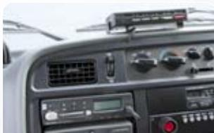
▶ Digital Travel Recorders are used to record idling times and other operational data.
