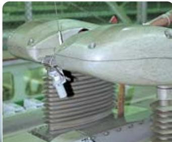
▶ Single pantograph trainsets require the technology to ensure constant contact between the overhead line and pantographs.
