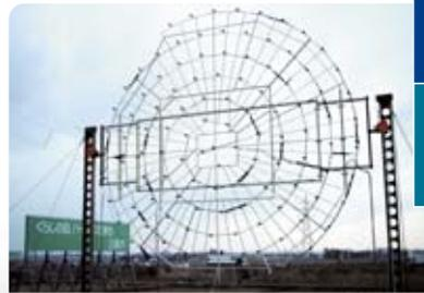
▶ A Spiral Array Microphone developed for precisely measuring noise sources; it received The Technology Development Award for 2004 from the Acoustical Society of Japan.
