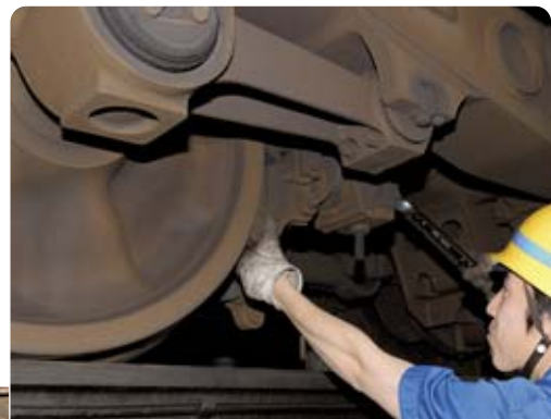
▶ Brake shoe(left: before use, right: after use) used to press against the wheel during braking and brake shoe replacement (above) at Mitaka Electric Car & Drivers Depot
