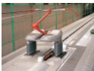
Single arm pantograph reduces wind noise
