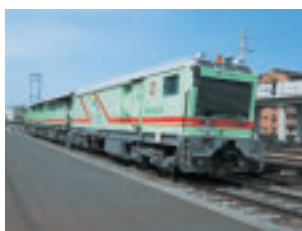
Rail alignment vehicle trims and flattens rails
