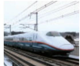
E2 series VVVF cars introduced on the Nagano Shinkansen Asama trains, and on Tohoku Shinkansen Hayate trains.
