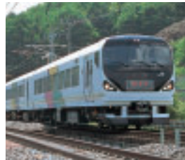
E257 series VVVF cars introduced on the Kaiji Express of the Chuo Line in FY 2001.
