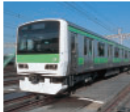
E231 series VVVF cars introduced on the Sobu Line (among others), and on the Yamanote Line in FY 2002.
