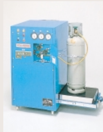
Equipment collecting CFCs and CFC substitutes used in trains
