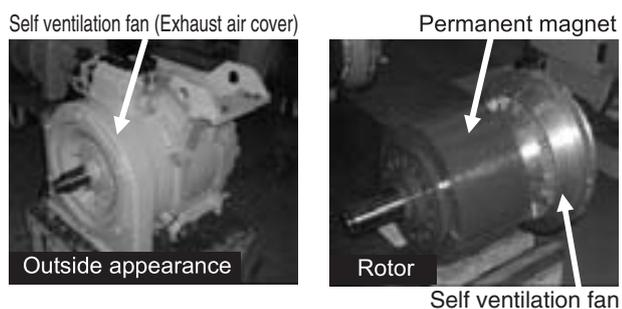
Fig.5: External appearance of synchronous motor and rotor
