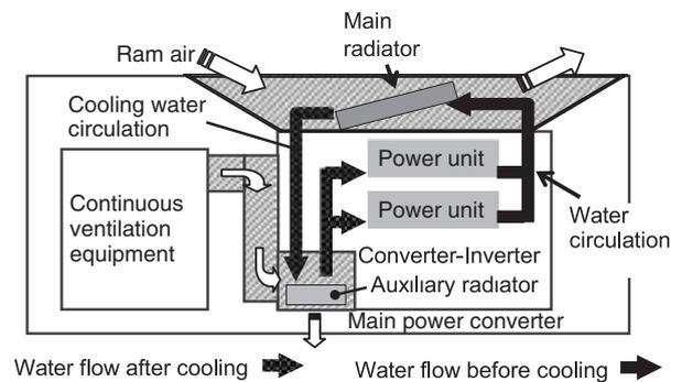
Fig.3: Illustration of cooling configuration
