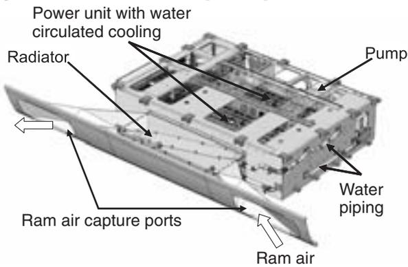
Fig.2: Ram air capture diagram
