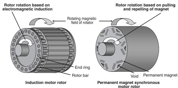
Fig.4: Principle of induction motor and synchronous motor operation
