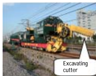
Fig. 10: New Ballast Excavation Machine
