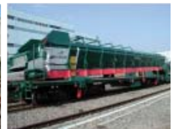
Fig. 11: Large Ballast Transporter
